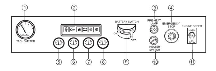
Figure 7. Engine Operating Panels
